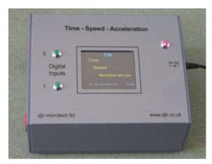
On the left hand side of TSA there are two digital input channels labelled 0 and 1. Each input can be via the DIN sockets or the 4mm sockets. Switches and light gates may be connected to these inputs. The DIN sockets are capable of supplying power to our light gates, sound switches etc.
