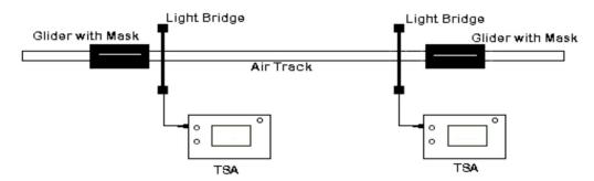
Do a trial run to show that each light bridge will be cut twice. Set up each TSA to measure two velocities. The data simply falls out in front of the students with the minimum of calculation being involved. Once the basic operation is understood, gliders of different mass can be used.
