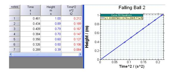
The slope of the  $s/t^2$  graph is a/2 and the results from this experiment give a value of the acceleration due to gravity as  $2 \times 4.74 = 9.48 \text{ m/s}^2$ .
