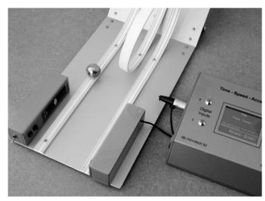
The Energy Track comprises two plastic tracks that run down a fixed slope and then along a horizontal section. A ball bearing placed on the slope will run down it and cut a light gate at the end of the track.
