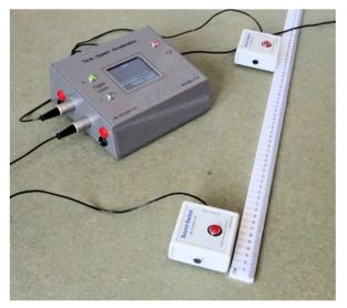
TSA can be used to measure the speed of sound. A typical setup using djb **microtech's** Sound Switches is shown.
